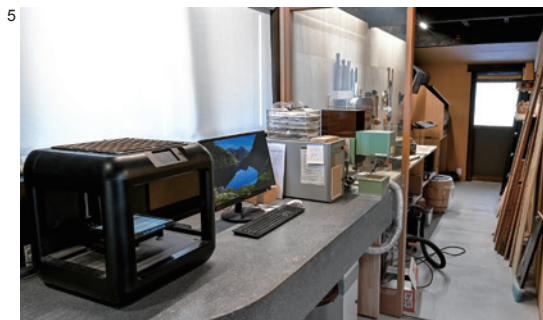
The green machine in the middle of IKEDA Terumasa's studio is a pulsed laser capable of cutting raden chips as fine as 0.2 mm. photo: NAKAGAWA Akifumi
